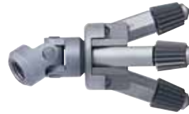
TYPE-4 Forward Swing Head Range: 1-3/4 in. (44.4 mm) - 4 1/4 in. (120.6 mm) Self feeding Deposit: 1/2 in. (12.7 mm) thick-soft to medium
