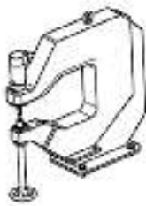
Assembly for riveting fastened to fixed frames examples
